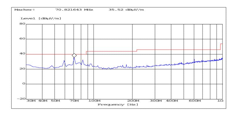
ANALYZER SETTINGS: RBW = 100KHz VBW = 100KHz
