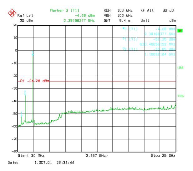
NOTE: The peak above the limit line is the carrier frequency.
