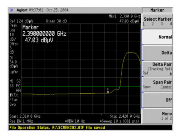
Detector mode: Peak Polarity: Horizontal
