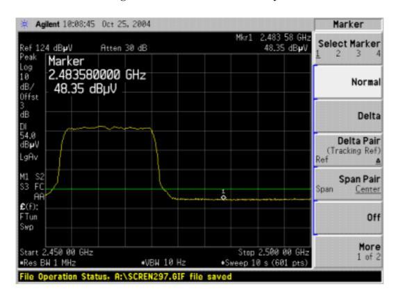
Detector mode: Peak Polarity: Horizontal
