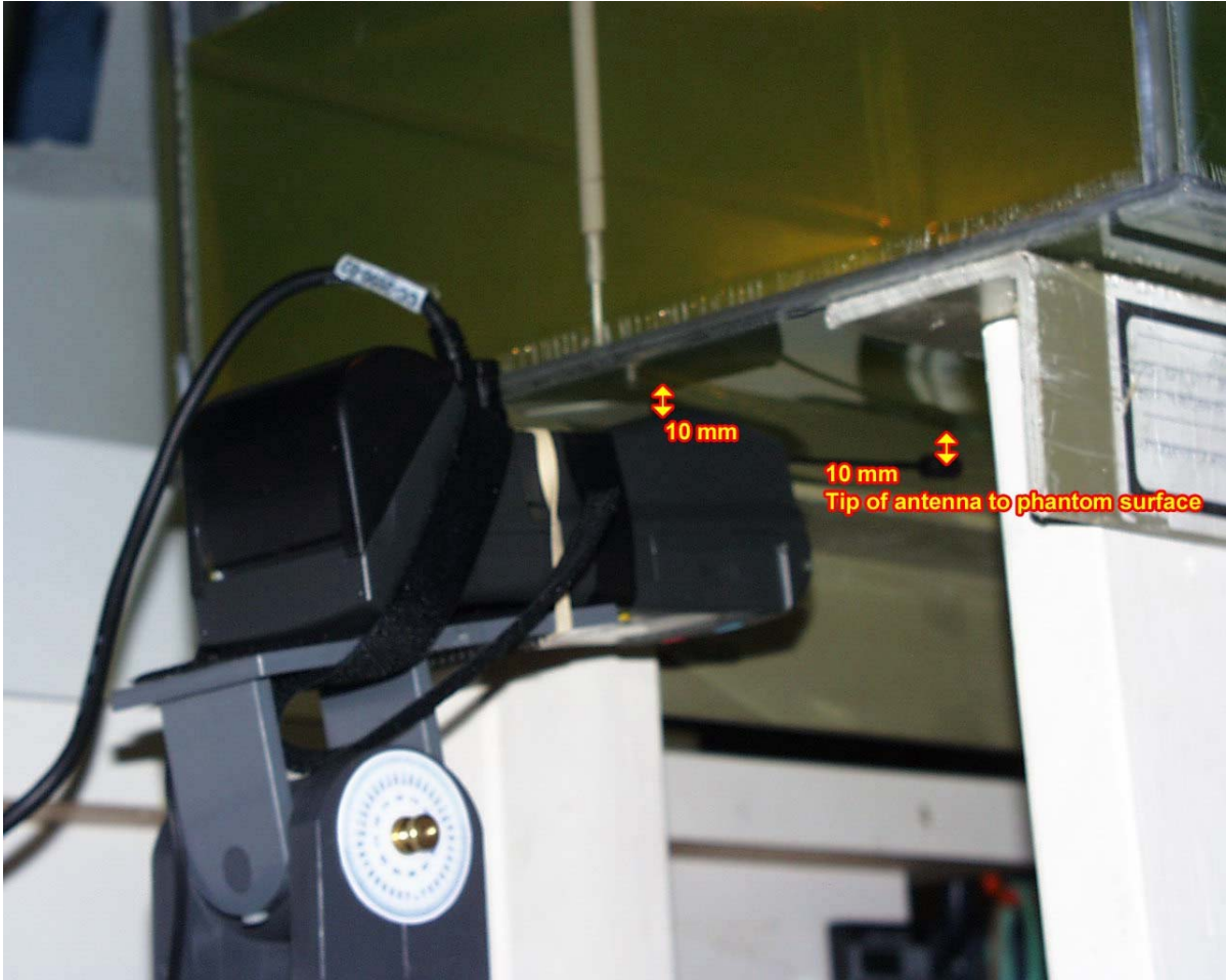
< Back side of EUT faced toward phantom, antenna fully extended and 10 mm separation >
