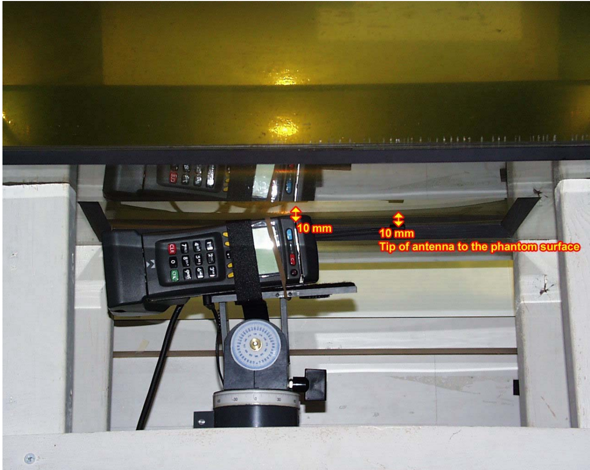
< Right side of EUT faced toward phantom, antenna fully extended and 10 mm separation >
