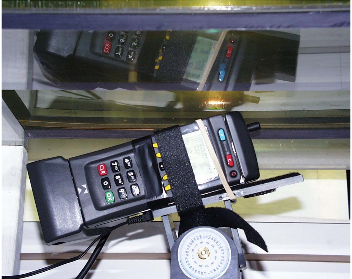
< Right face toward phantom, tip of antenna in contact and antenna fully retracted >
