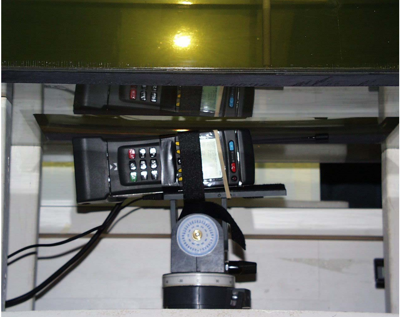
< Right face toward phantom, the tip of antenna in contact and antenna fully extended >
