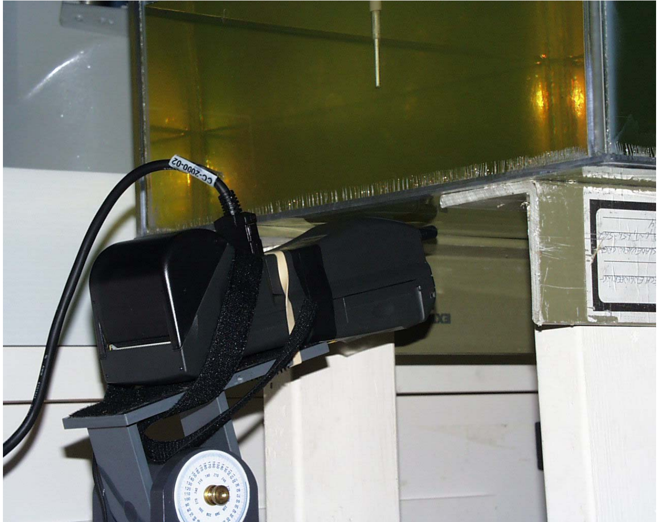
< Back face toward phantom, the tip of antenna in contact and the antenna fully retracted >
