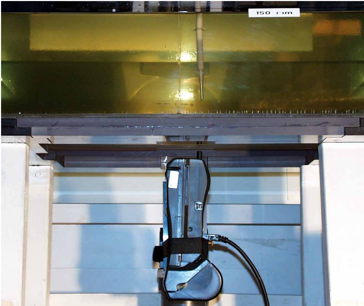
< D.U.T perpendicular to the phantom with spacing of 15 mm and the antenna fully retracted >
