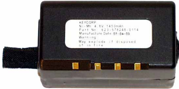
< Rechargeable Ni-MH battery pack (Keycorp, P/N: 623-578248-0114, 4.8 VDC, 1450 mAh) >
