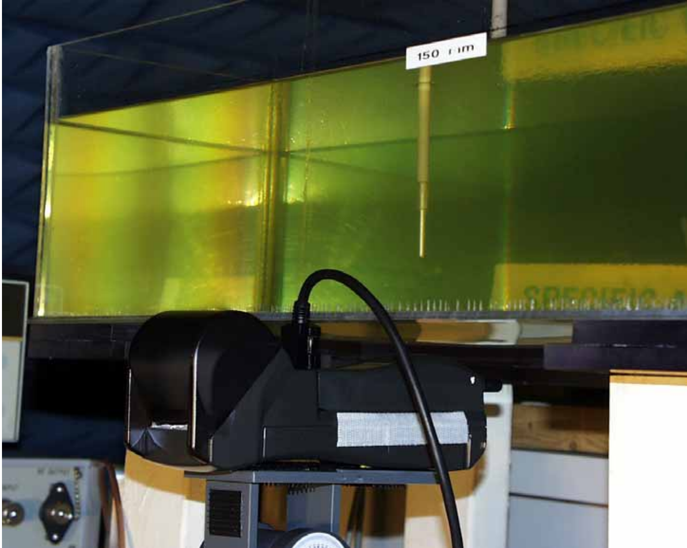
< Back-face in parallel to the phantom with spacing of 15 mm and the antenna fully retracted >
