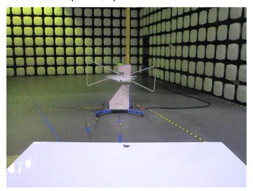
Radiated Emissions (above 1GHz) & Radiated Emissions which fall in the restricted bands
