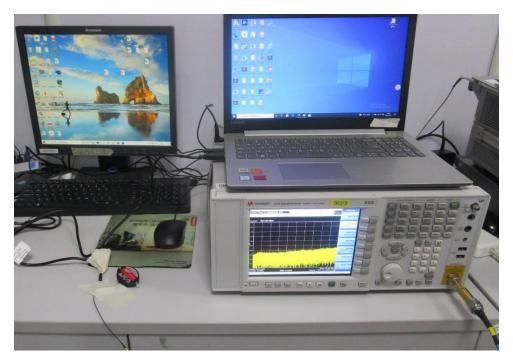
Emission Mask & Radiated Emissions (9kHz-30MHz)
