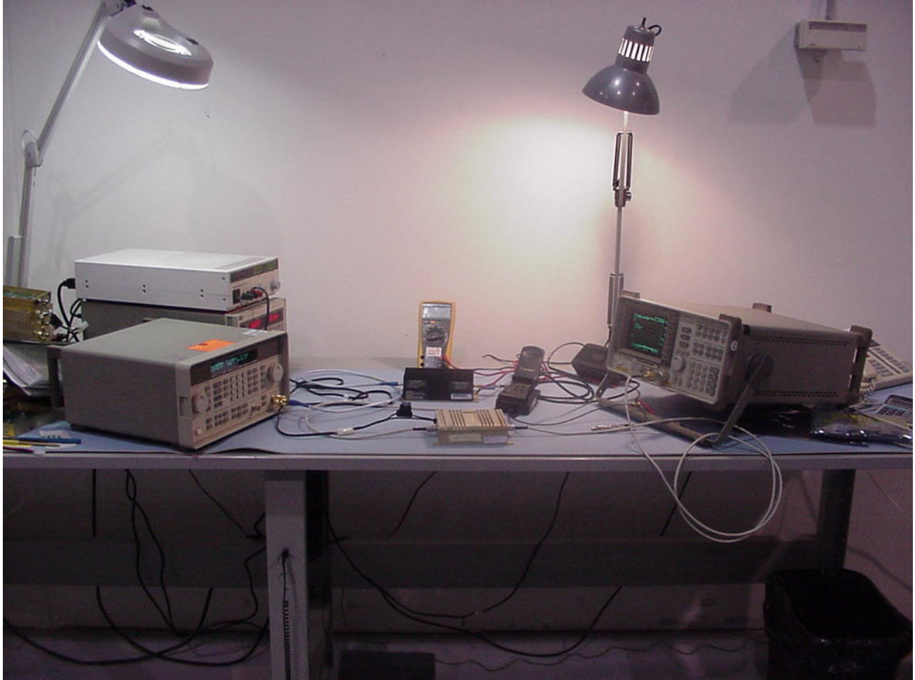
Picture B-3: EUT Set-up for Bench Top, Conducted Emissions, Power Output Testing.
