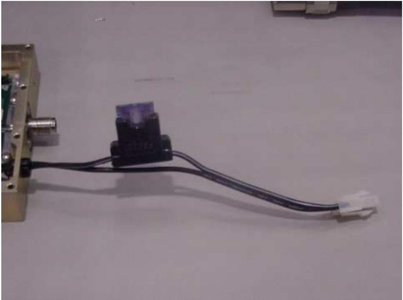
Picture B-6 SG800 DC Power Cable with 3-Amp Fuse
