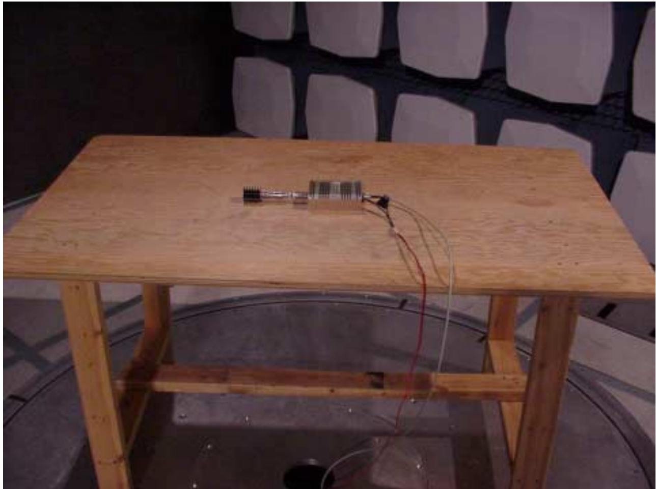
Picture B-1: EUT Set-up in 3-meter Anechoic
