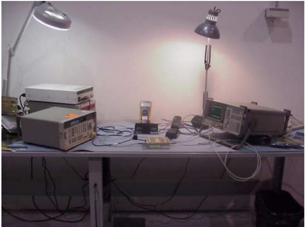
Picture B-3: EUT Set-up for Bench Top Testing, For Conducted Emissions, Power Output Testing.
