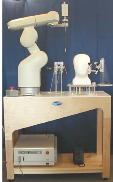
Figure 6: Principal components of the SAR measurement test bench
