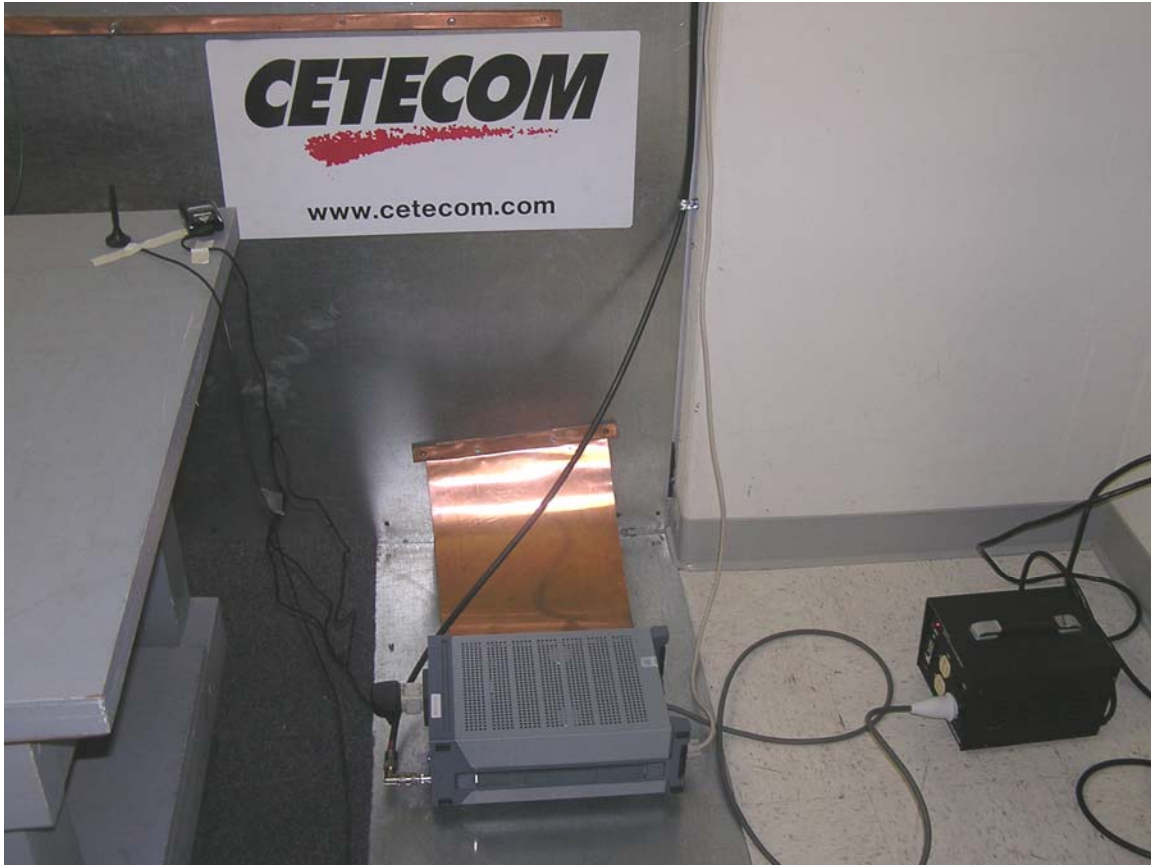
Test setup – AC Line Conducted Emissions
