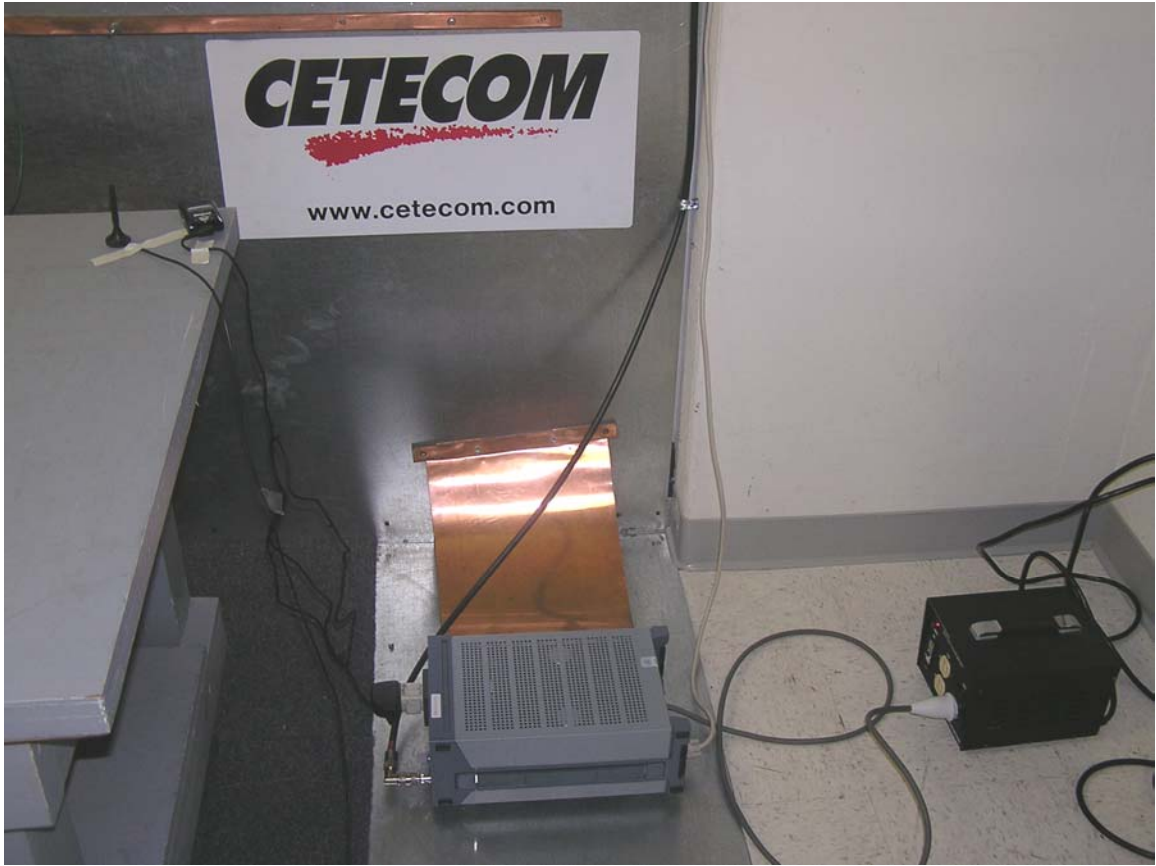
Test setup – AC Line Conducted Emissions
