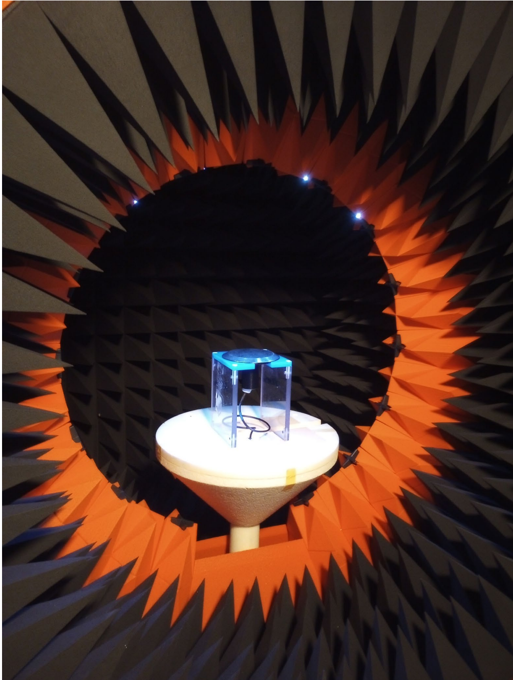
Figure 2 - Antenna Under Test in StarLab system
