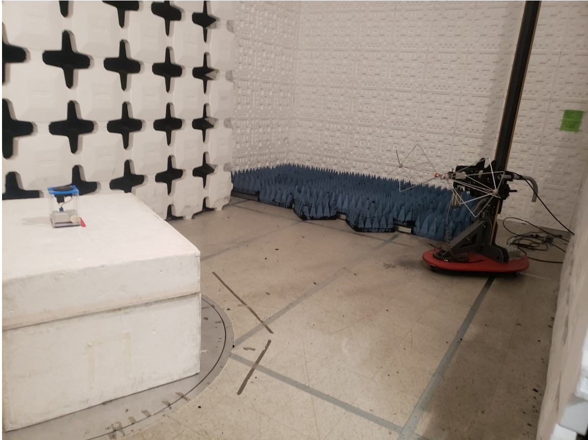
Figure 2. Radiated Emissions 30-1000 MHz
