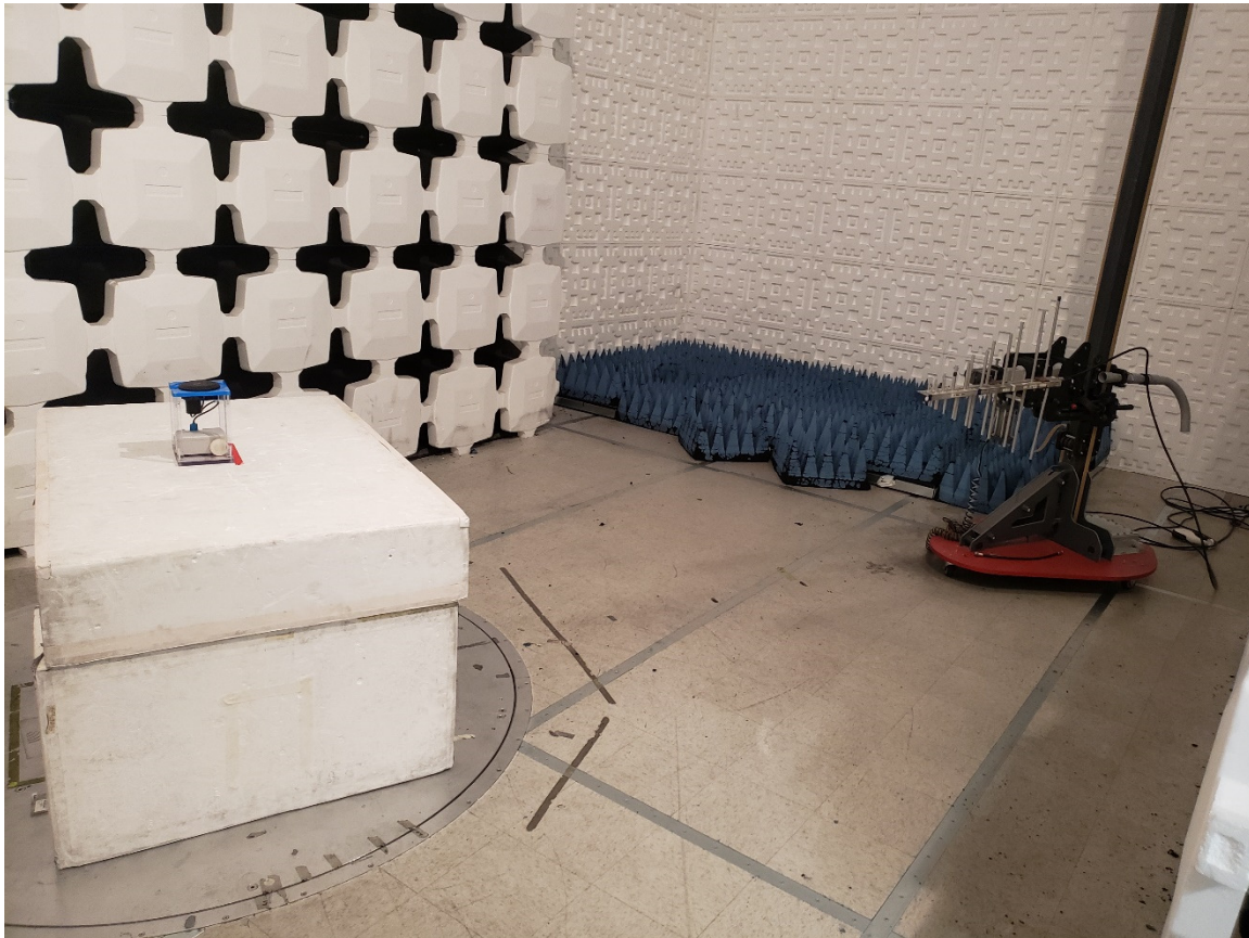
Figure 3. Radiated Emissions, 200-1000 MHz
