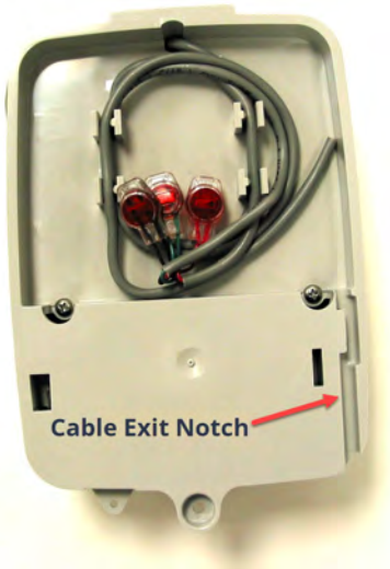
Figure 17 – Cable Exit Notch
