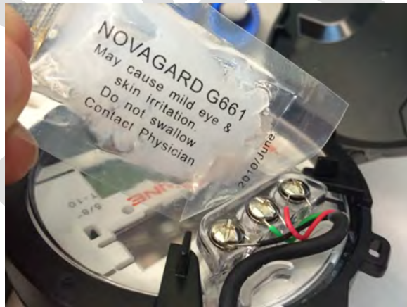
Figure 8 – Application of the Sealant
