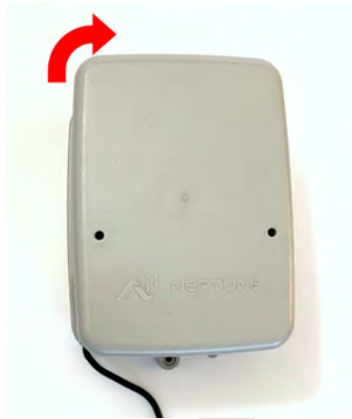
Figure 19 – Swiping the R900 cellular endpoint
