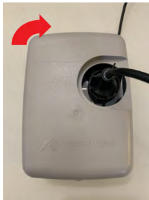
Figure 35 – Swiping the R900 cellular endpoint
