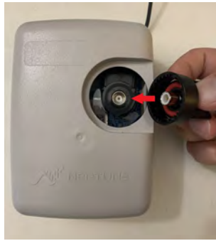
Figure 32 – R900 cellular endpoint Conductor Pin
