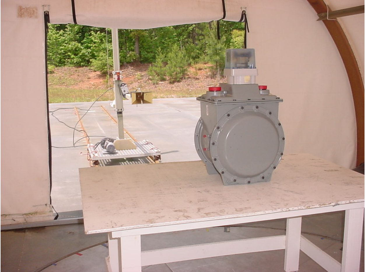
Figure 7: Test Setup – Radiated Emissions – Actaris Model 675A
