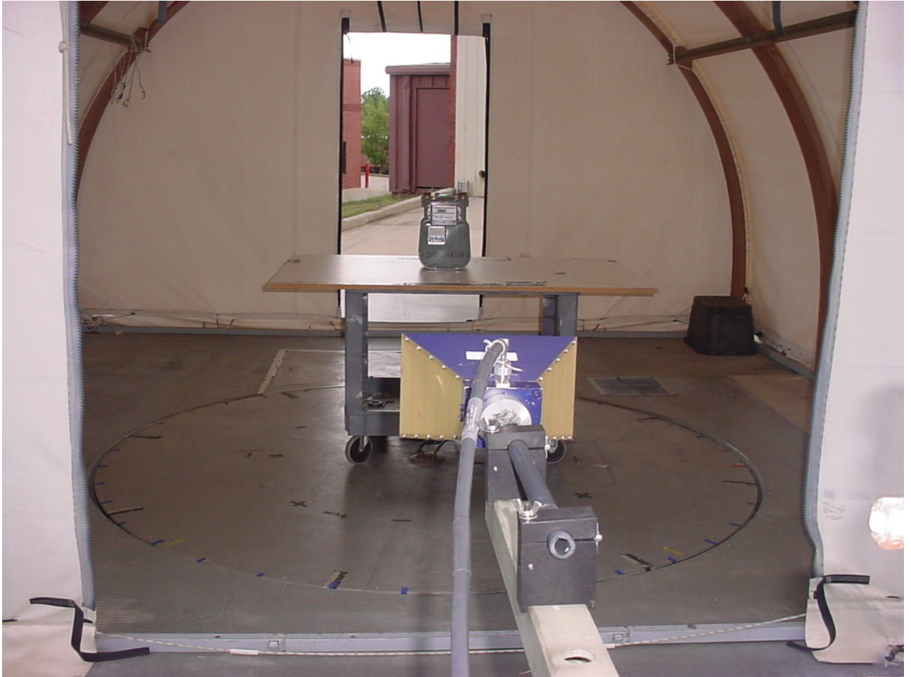
Figure 2: Test Setup – Radiated Emissions – American Meter Company Model AC-250
