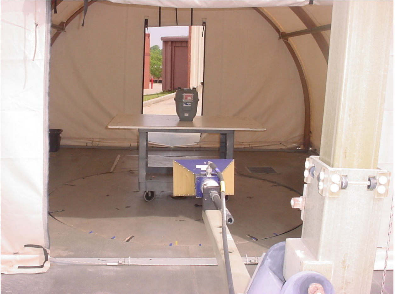
Figure 6: Test Setup – Radiated Emissions – Sensus Metering Systems Model R-275
