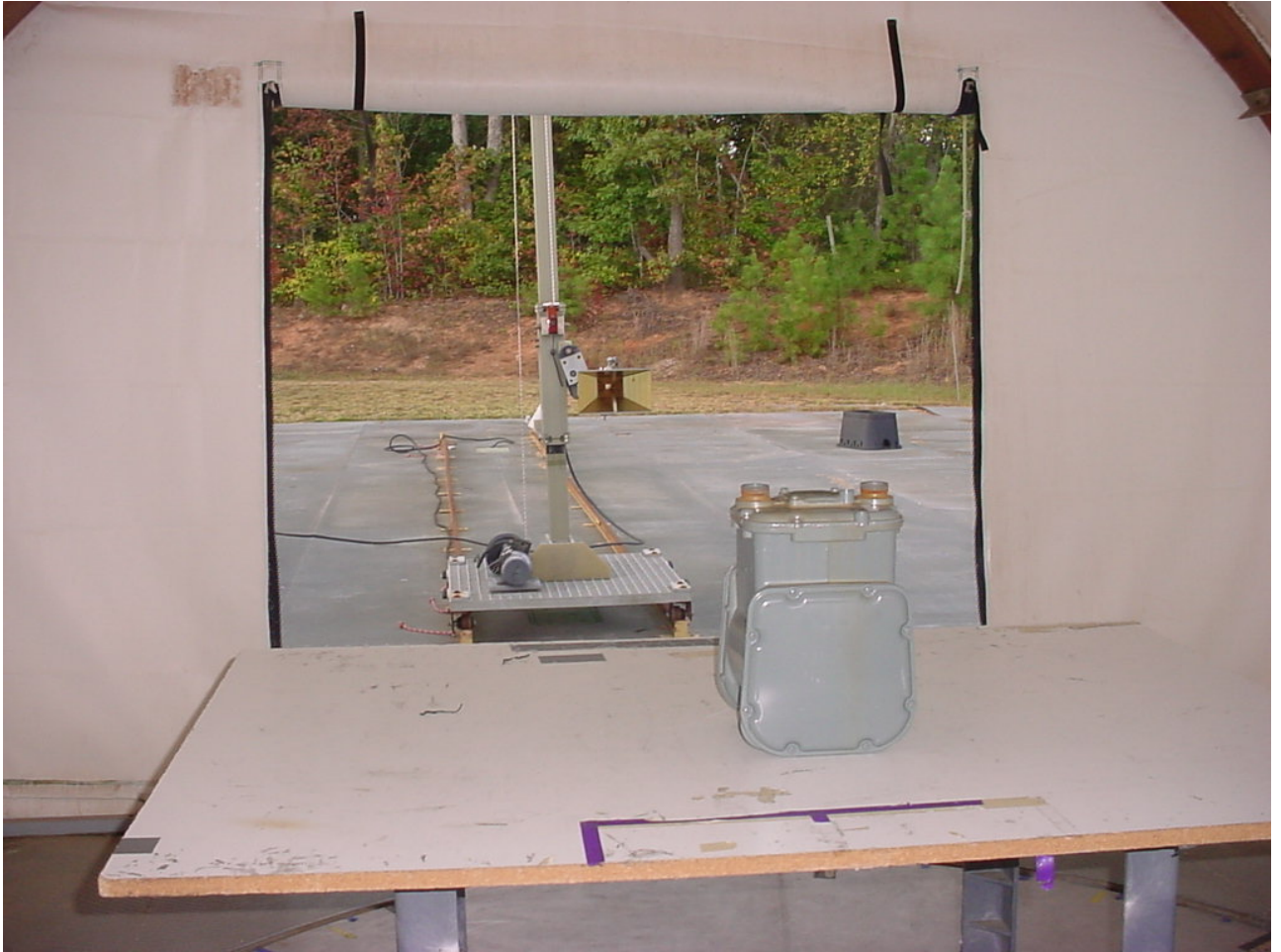
Figure 1: Test Setup – Radiated Emissions – American Meter Company Model AC-250
