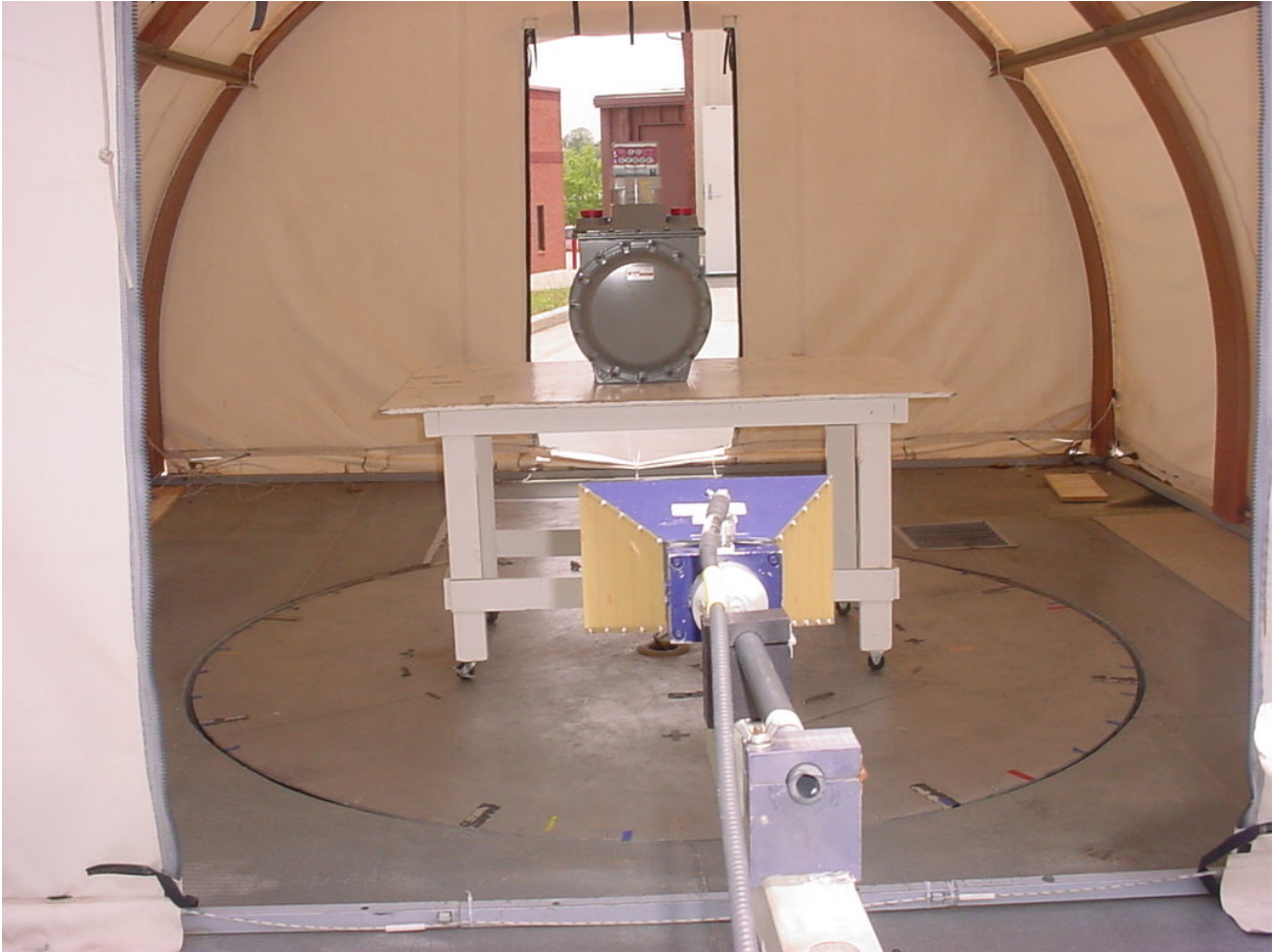
Figure 8: Test Setup – Radiated Emissions – Actaris Model 675A
