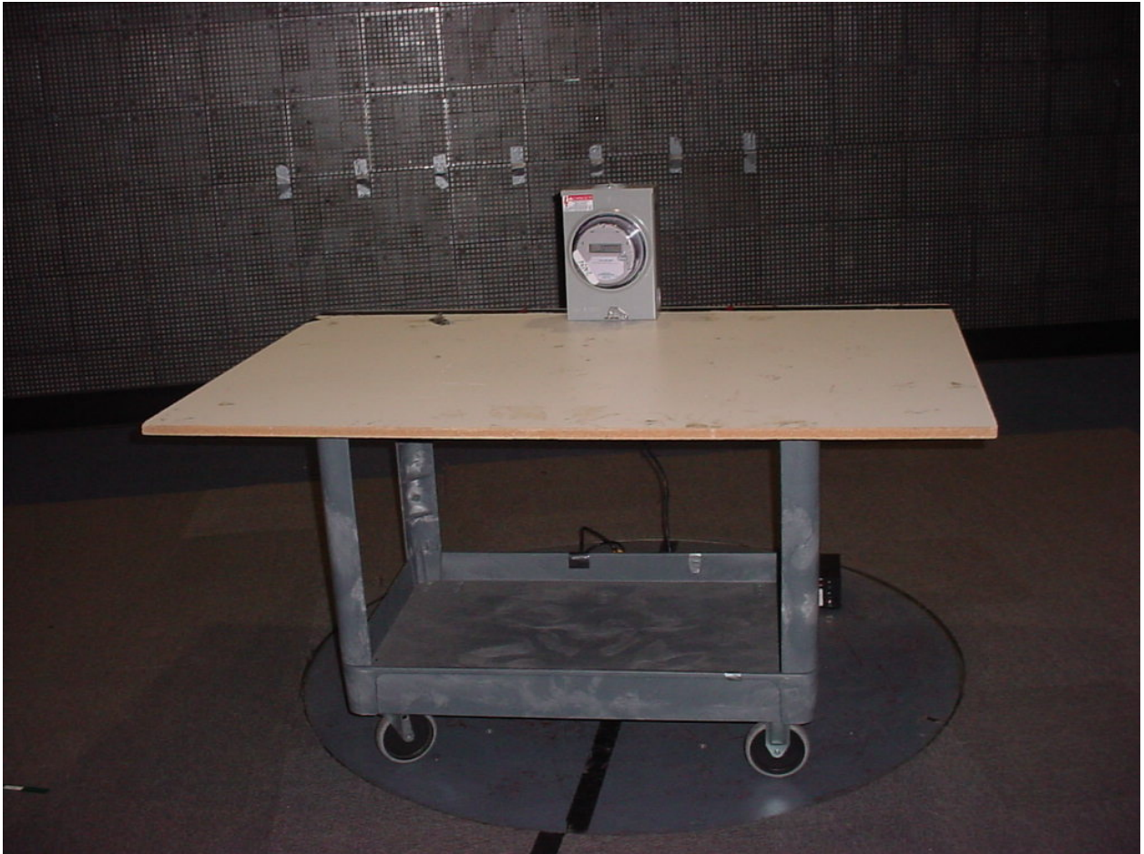
Figure 1: Test Setup – Radiated Emissions – Front View
