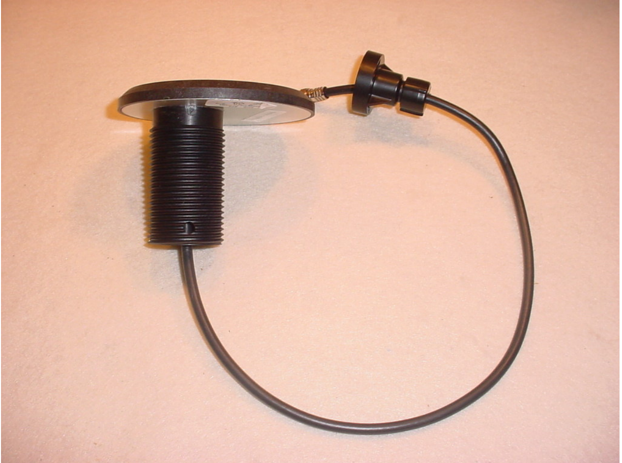
Figure 6: - External Photos – Pit Mount Patch Antenna
