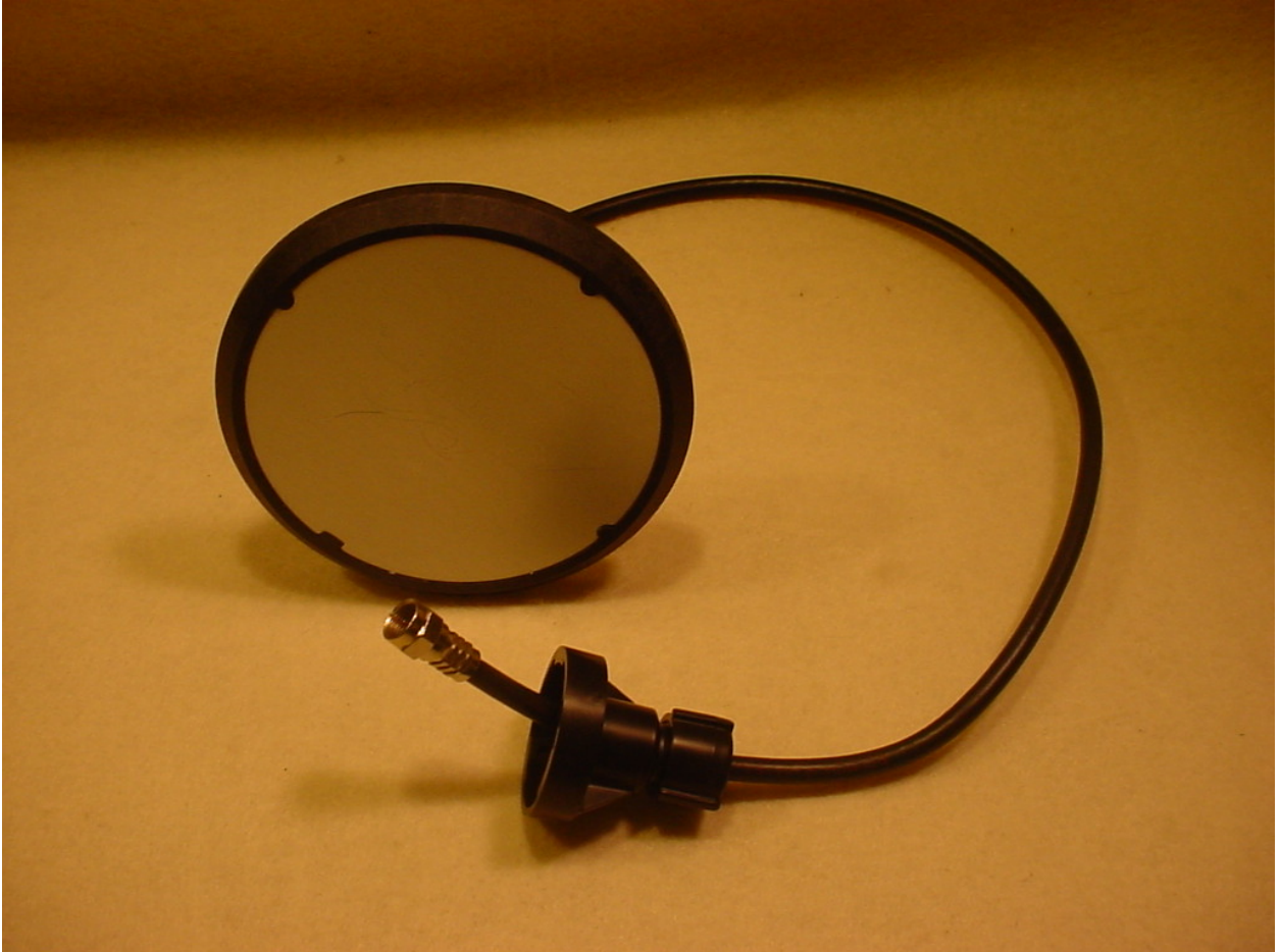
Figure 7: - External Photos – Pit Mount Patch Antenna
