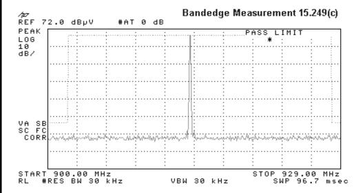
Note 1: No correction factors applied to measurement above. Maximized Fundamental signal. A lower Resolution and Video bandwidth was used to provide more dynamic range for the 50-dB attenuation requirement.
