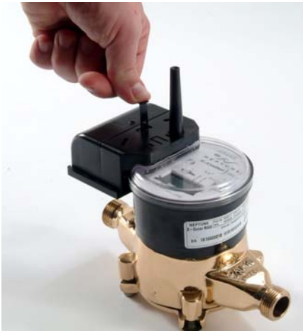
Figure 9 Pushing in New Tamper Nail
