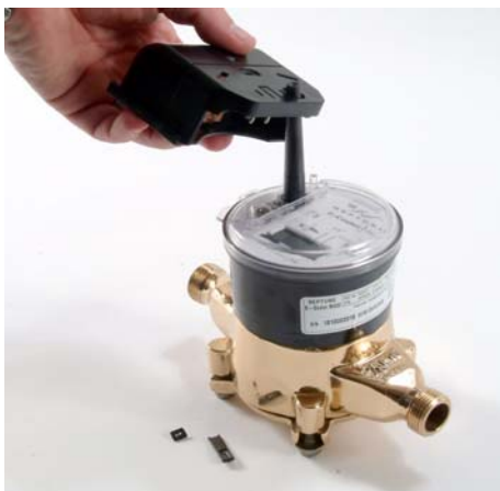
Figure 8 Sliding Battery over Antenna
