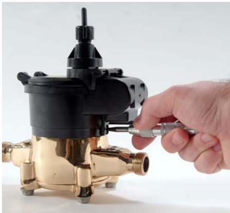
Figure 10 Screwdriver in Seal Pin
