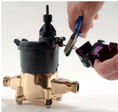
Figure 12 Cutting the Battery Wires
