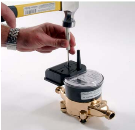
Figure 7 Screwdriver in Tamper Nail
