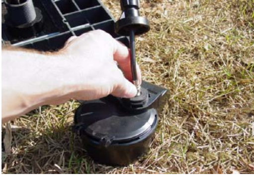
Figure 16 Connecting the Coaxial Cable
