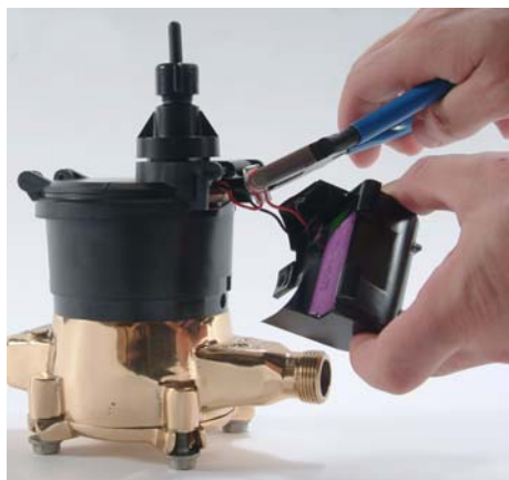
Figure 13 Using Scotchlok to Splice Wires
