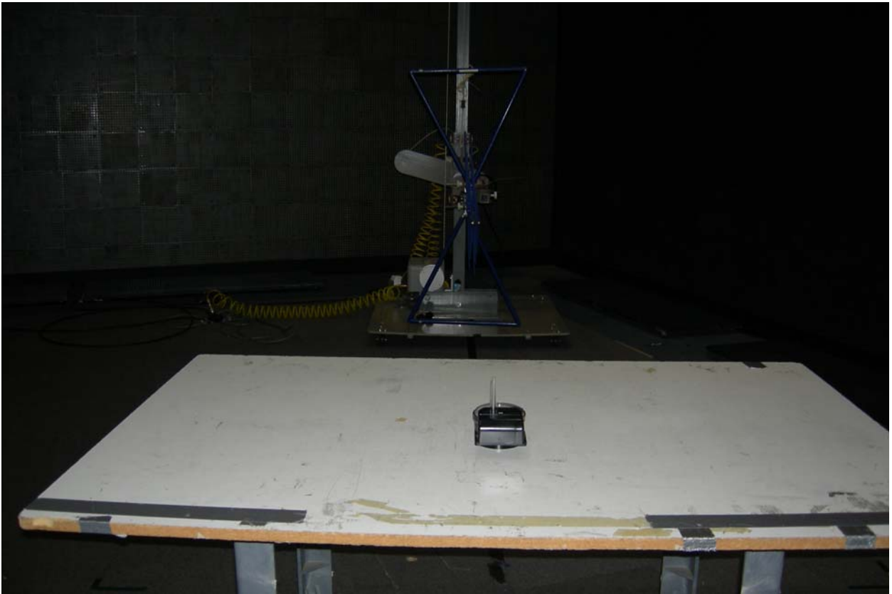
Figure 4: Test Setup – Radiated Emissions – Unintentional Basement Configuration
