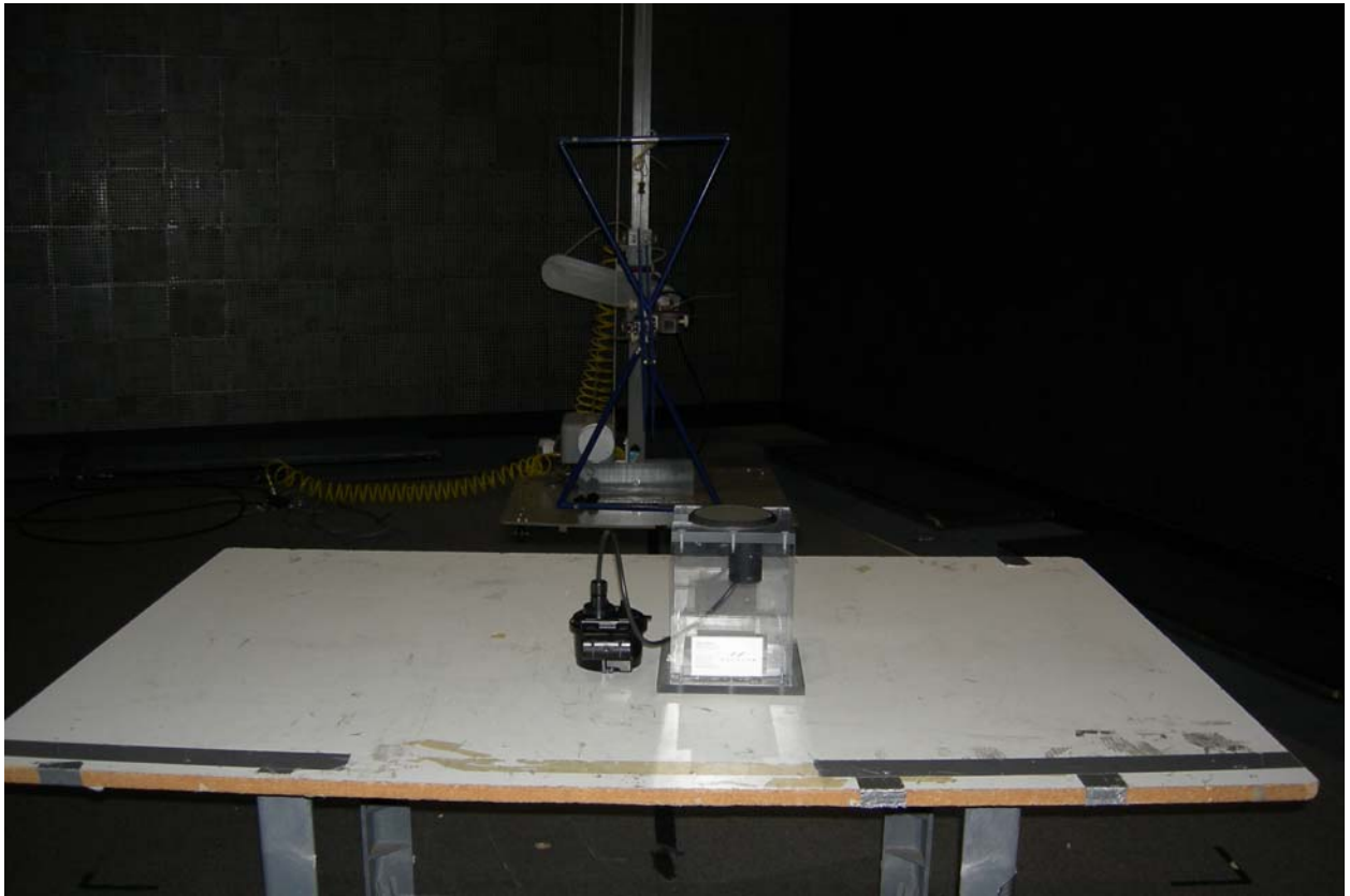
Figure 5: Test Setup – Radiated Emissions – Unintentional Pit Patch Configuration
