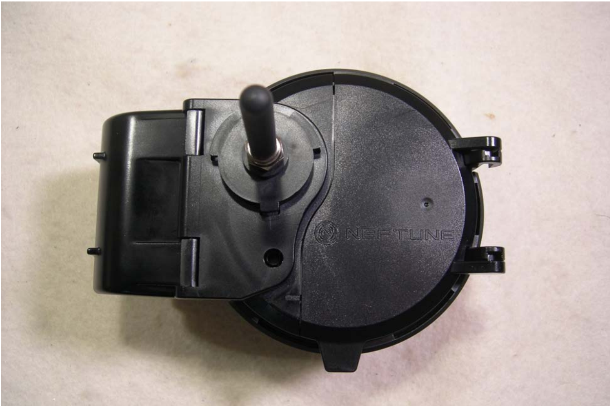
Figure 8: Pit Version (Slip on Monopole Antenna) – Top
