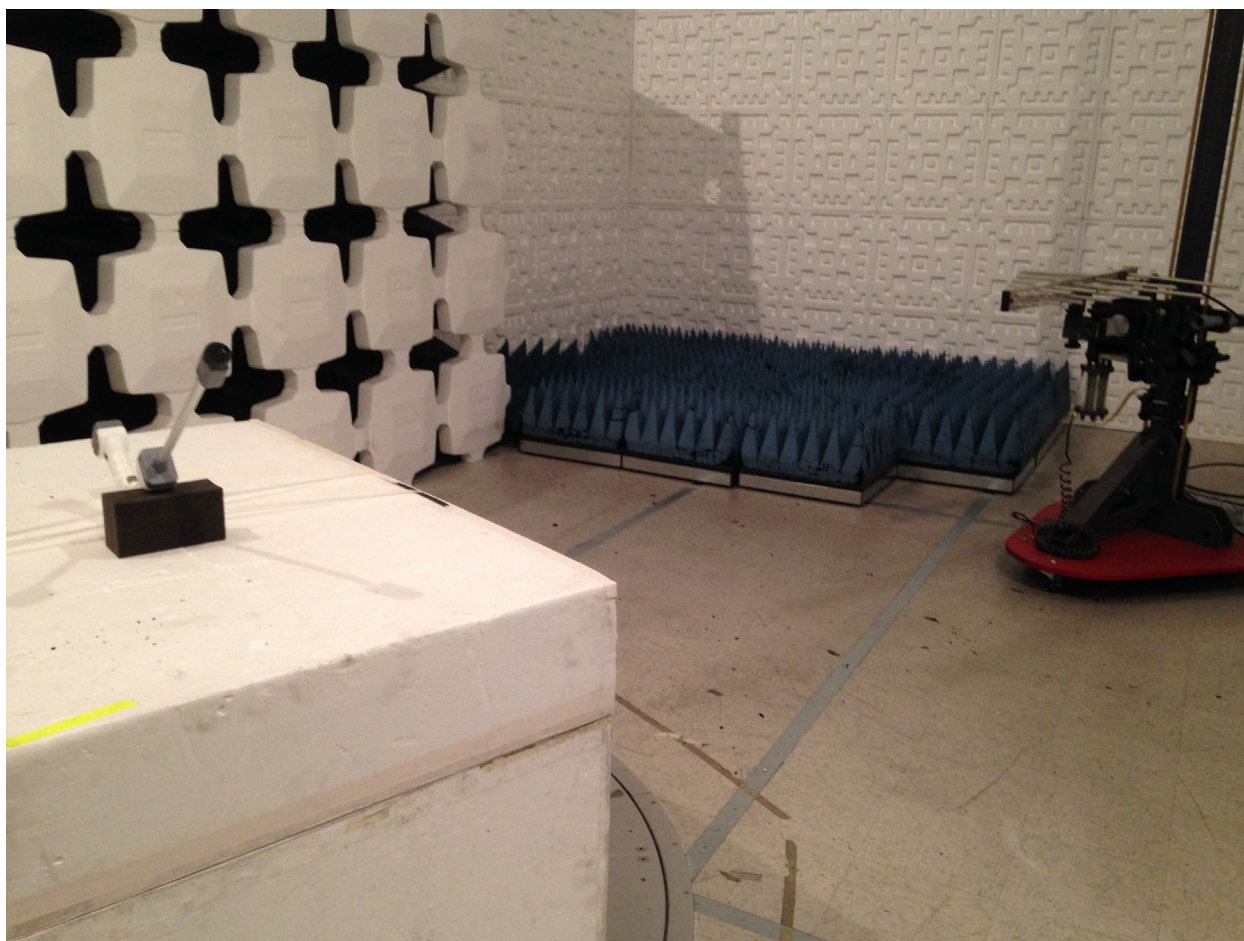
Figure 4. Radiated Emissions, 200-1000 MHz
