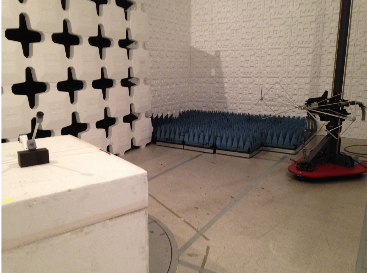
Figure 3. Radiated Emissions, 30-200 MHz
