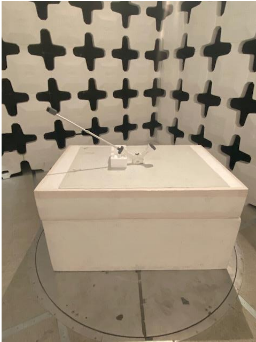
Figure 1. Radiated Emissions Test Setup
