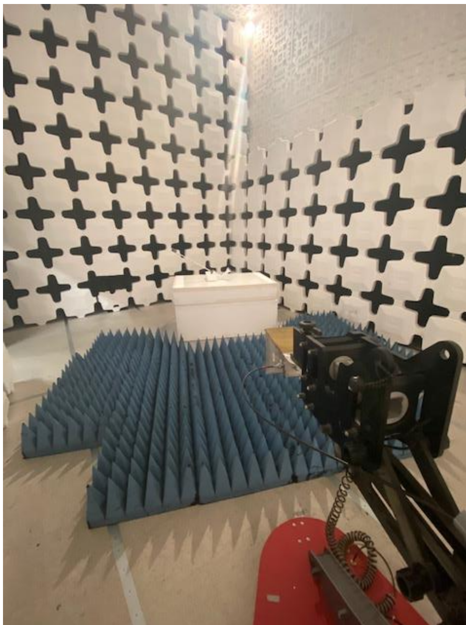
Figure 4. Unintentional Radiated Emissions Test Configuration (Above 1 GHz)
