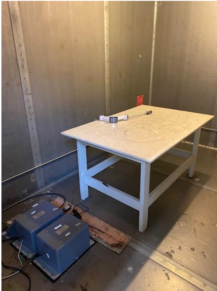
Figure 6. Power Line Conducted Emissions Test Setup.
