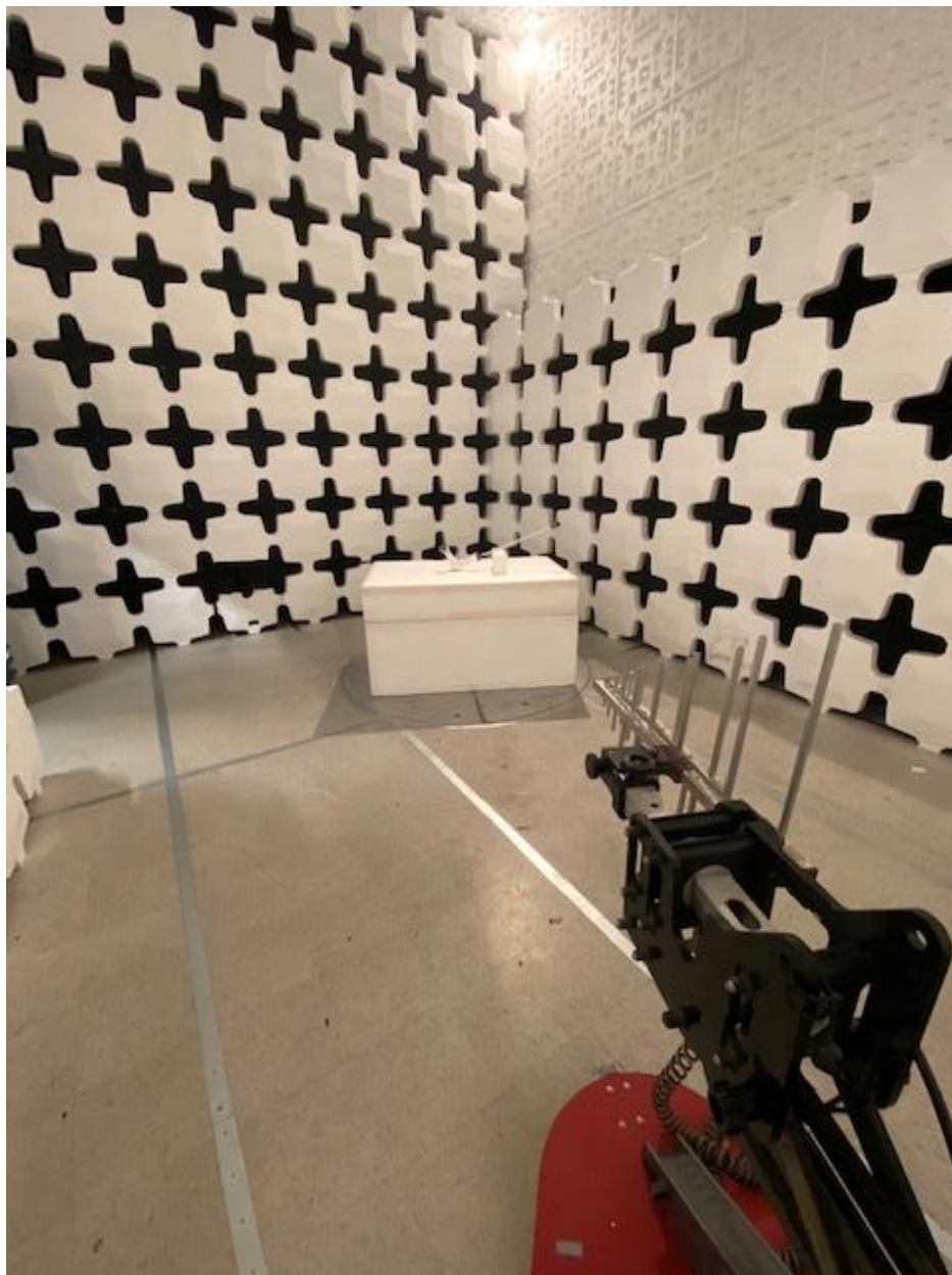
Figure 3. Radiated Emissions Test Configuration (200 MHz to 1 GHz)
