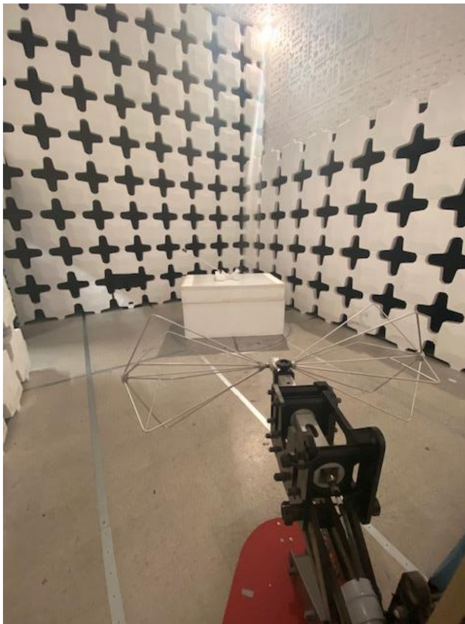
Figure 2. Radiated Emissions Test Configuration (30-200 MHz)
