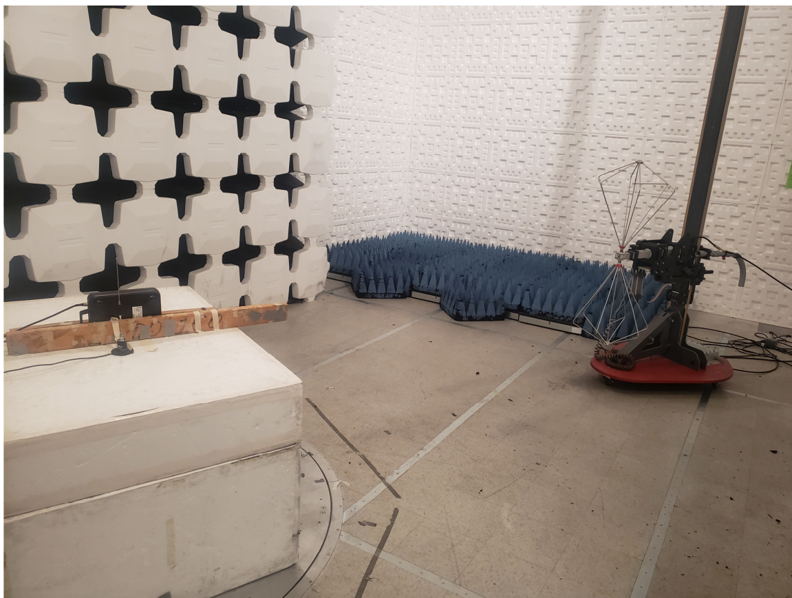
Figure 2. Radiated Spurious Emissions, 30 - 200 MHz
