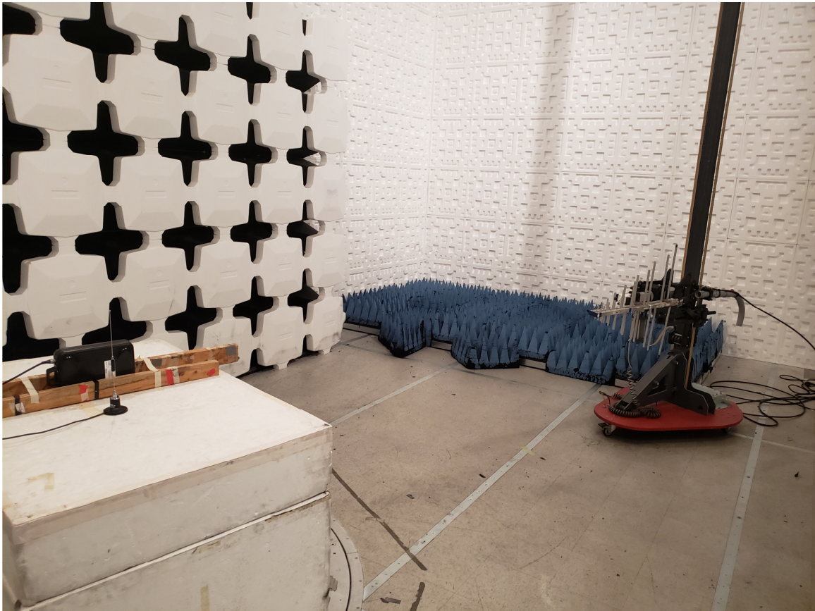
Figure 3. Radiated Spurious Emissions, 200 - 1000 MHz
