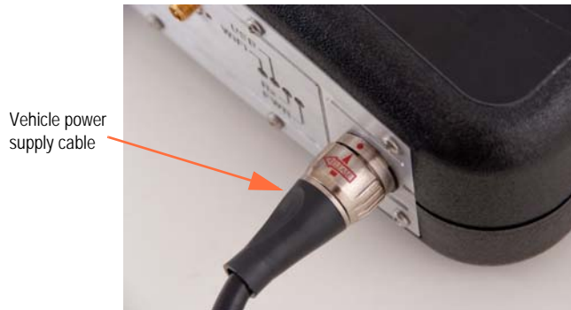
Figure 3.16 Vehicle Power Supply Power Cable
