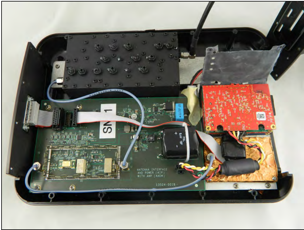
Figure 3: Internal Photo – MRX920v3 Assembly – Screws Removed Holding Foil Shield to Power PCBA in Board Stack, Foil Shield Lifted
