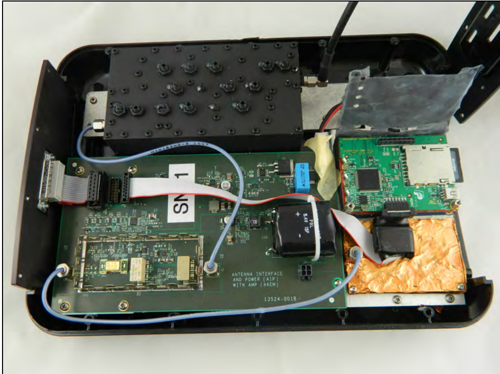
Figure 4: Internal Photo – Power PCBA Removed From Board Stack Showing I/O PCBA (Top), Foil Shield Lifted
