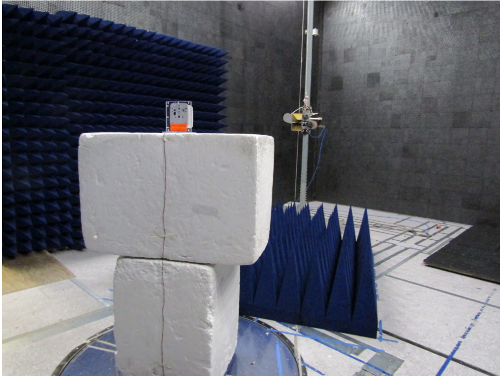
Figure 7: Equipment Under Test – Radiated Emissions >1GHz (Wall Mount)
