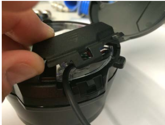
Figure 9 – Covering the Terminal Screws
