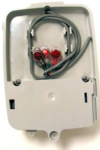
Figure 15 – Cable in Back of Mounting Adapter
