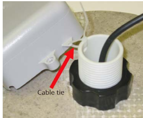
Figure 43 – Attaching the CMIU™ to the Antenna Shaft
