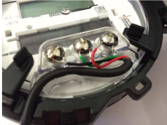
Figure 7 – Cable Threaded Around Strain Relief Posts
