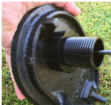
Figure 30 – Antenna Installation Complete
