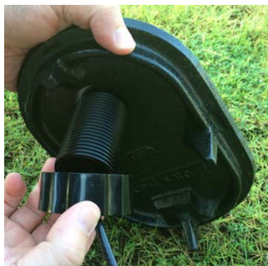
Figure 29 – Locking the Nut on the Antenna
