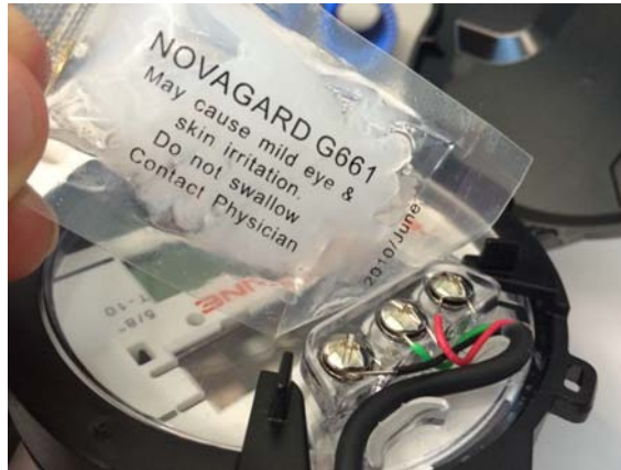
Figure 5 Application of the Sealant
