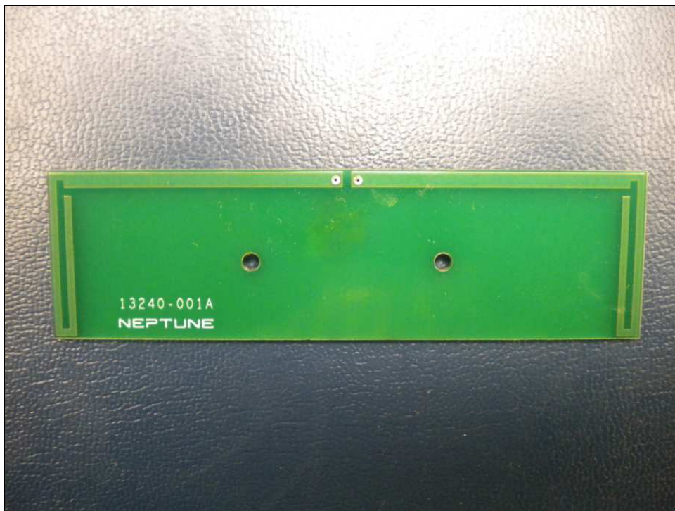
Figure 13: Internal Photo – 900 MHz Receiver Antenna Board
