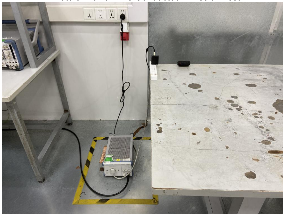
FCC ID: P2F-FD9970 Photo of Power Line Conducted Emission Test
