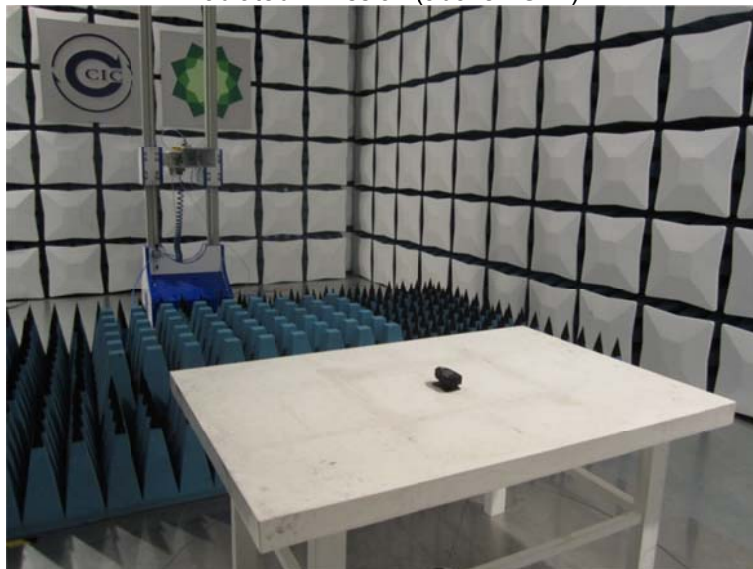
Radiated Emission (above 1GHz)
