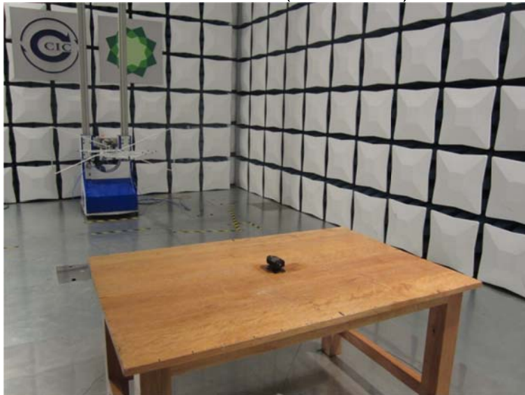
Radiated Emission (above 1GHz)
