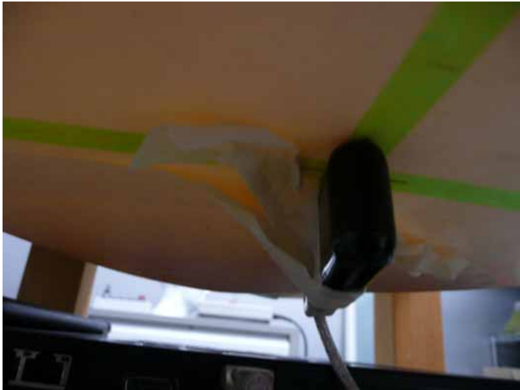
The Vertical-Back of the EUT to the flat phantom distance 5mm. EUT Orientation D of EUT Position
