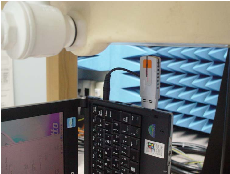
Fig.3 Photograph of the antenna tip is upward and at a distance of 1.5 cm from the base of the phantom.
