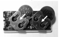
Use care when installing the battery and observe the correct polarity when the battery is inserted. Use only CR2032 batteries for replacement.
