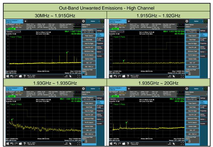
Note 1: The BS spurious out-of-band transmission level is below the indicated limit.
