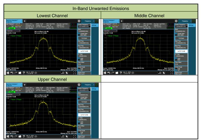
Note: The BS spurious in-band of Middle Channel transmission level is below the indicated limit.
