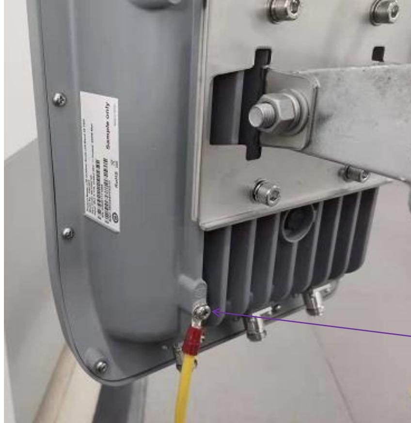
Grounding screw on the device
