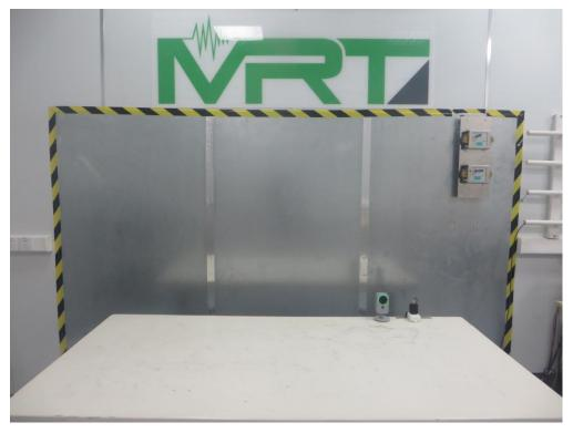
Test Mode: Mode 1 Description: Back View of Conducted Emission Test Setup For Power Port
