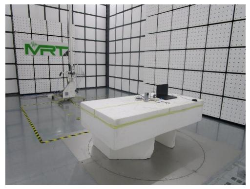
Test Mode: Mode3 (Adapter: PSAF10A-050Q) Description: Radiated Emission Test Setup for below 1GHz
