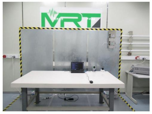
Test Mode: Mode3 (Adapter: 1A52-UB52A) Description: Back View of Conducted Emission Test Setup
