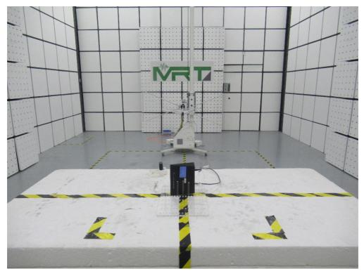
Test Mode: Mode 1 Description: Radiated Spurious Emission Test Setup for 1GHz ~ 18GHz
