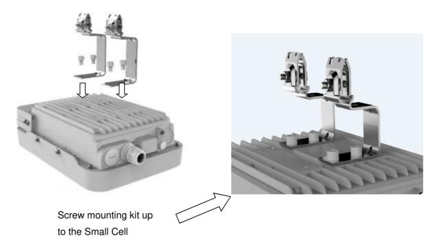
Make strand through mounting kit clamps and then screw the bolts on the clamps to lock the strand. Finally, it will look like below:
