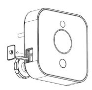
2. Insert the micro SD card into the slot.
