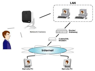
Figure 1: Network Diagram - Waterproof HD IP Camera
