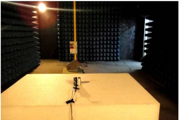
**Powerline Conducted Emissions Setup Photos**
