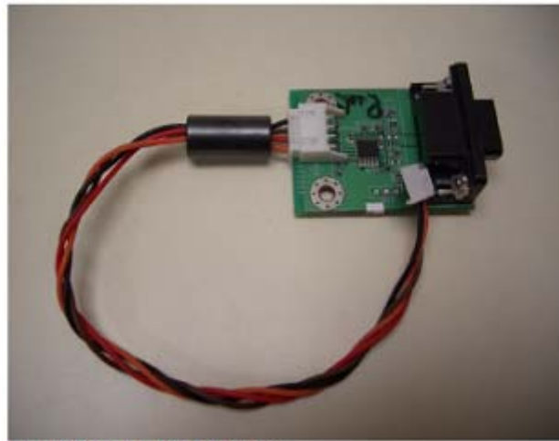
Platform debugging cable
