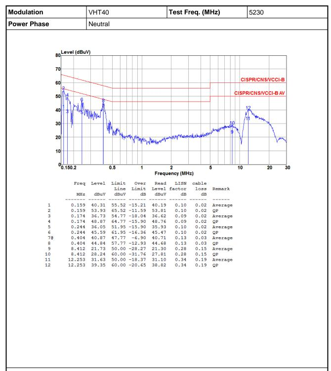
Note 1: Level (dBuV) = Read Level (dBuV) + LISN Factor (dB) + Cable Loss (dB).
