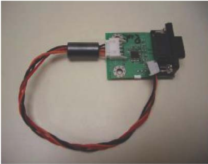
Platform debugging cable
