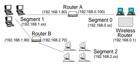
Figure 43: Routing Example
