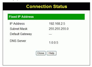
Figure 46: Connection Details - Fixed IP Address
