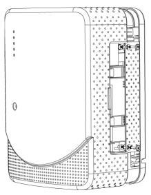
**Note:** Use a screwdriver to remove the two screws of the battery cover before installing the battery.
