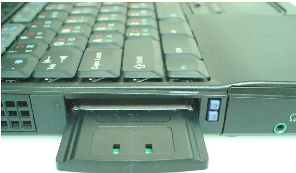
Fig.11 With IBM ThinkPad T30 PCMCIA slot
