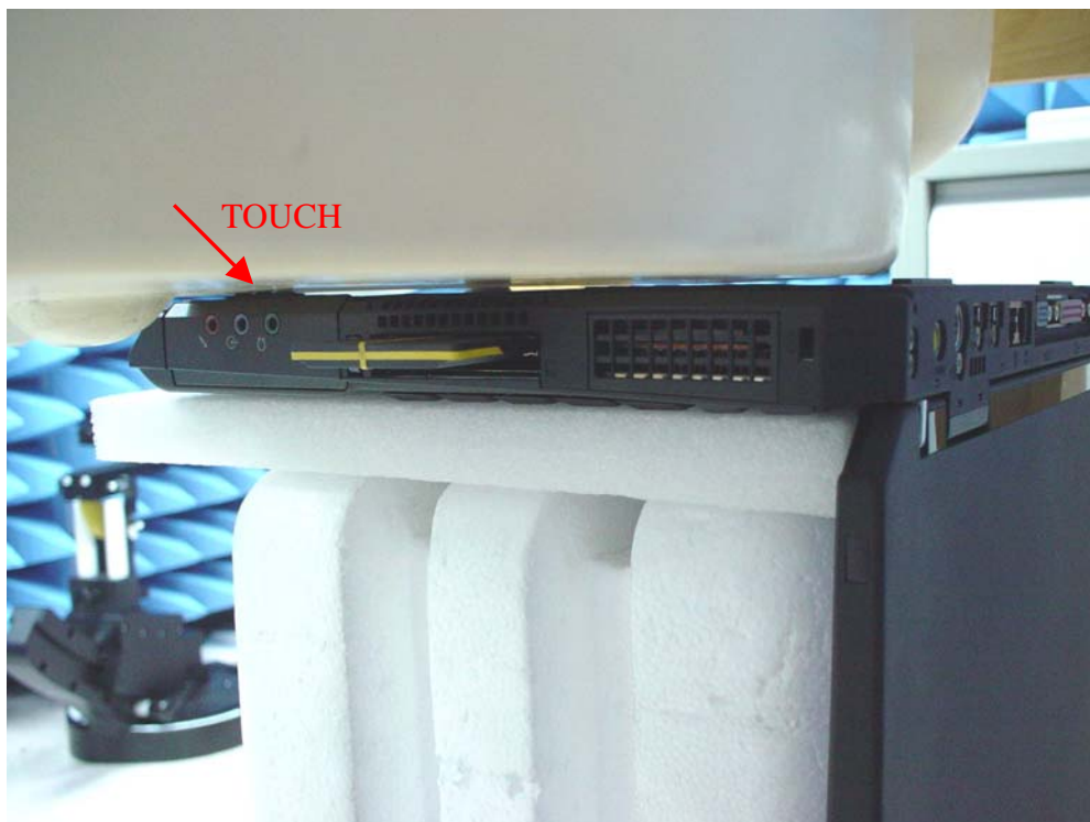
Fig.6 Photograph of the Bottom of the Pc is paralleled and at a distance of 0.0 cm from the base of the phantom.
