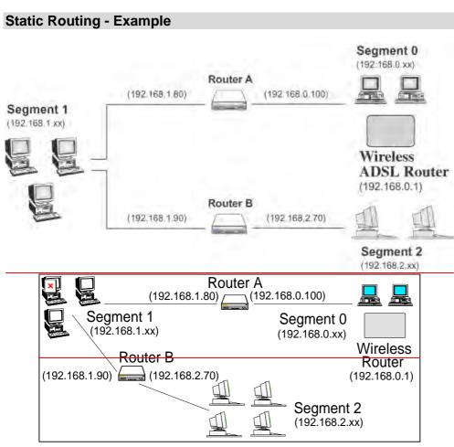
Figure 69: Routing Example
